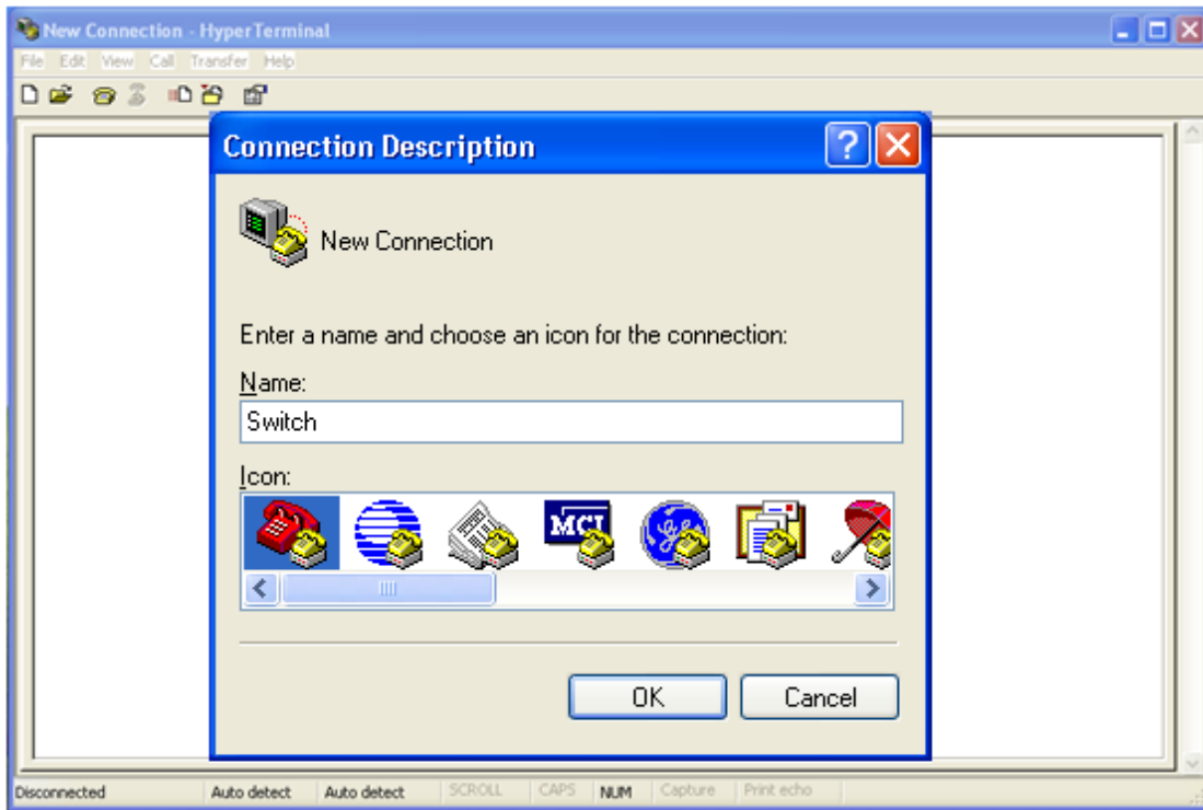
Figure 2 Creating a New Connection
