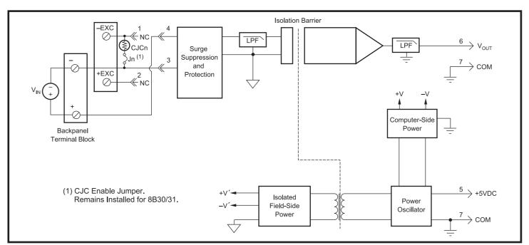
Figure 1: 8B30/31 Block Diagram
