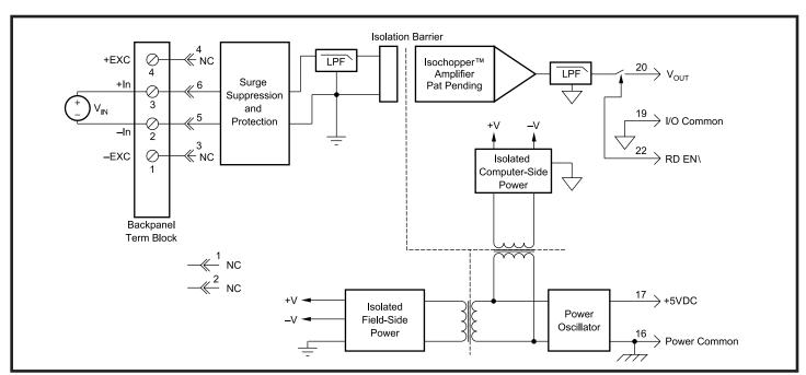
Figure 1: SCM5B30/31 Block Diagram
