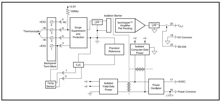
Figure 1: SCM5B37 Block Diagram
