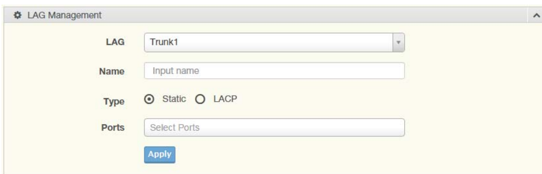
Figure 4.20 L2 Switching > Link Aggregation > LAG Management
