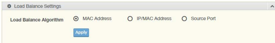
Figure 4.19 L2 Switching > Link Aggregation > Load Balance
