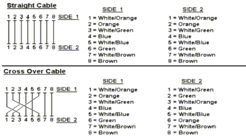
Figure A-1: Straight-Through and Crossover Cable
