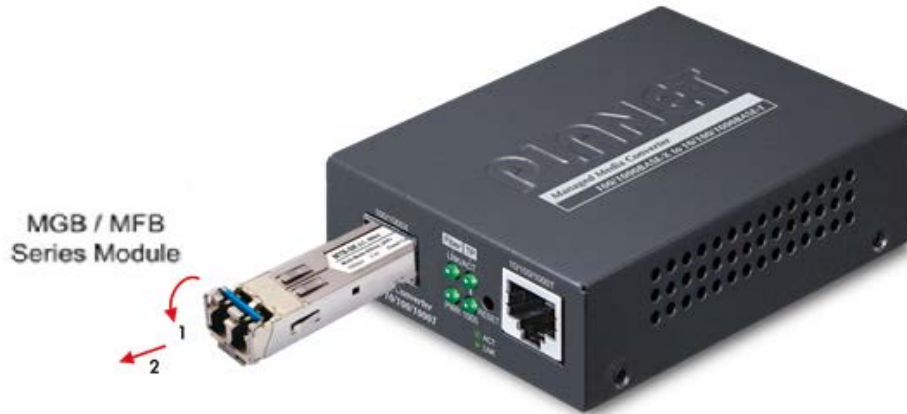
Figure 2-4: How to Pull Out the SFP Transceiver
