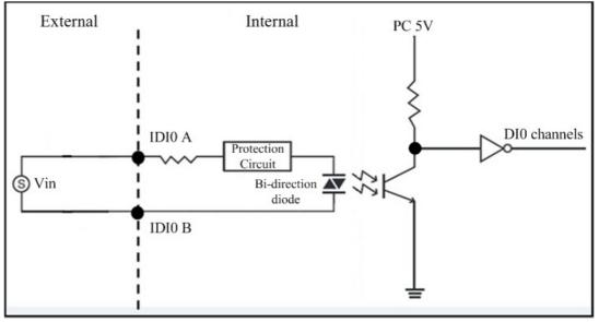
Figure 3.1 Isolated Digital Input Connections
