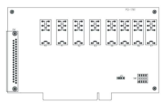
Figure 2.1 Card Connector, Jumper and Switch Locations
