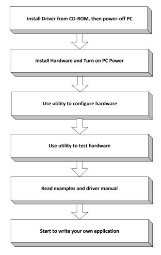
Figure 1.1 Installation Flow Chart
