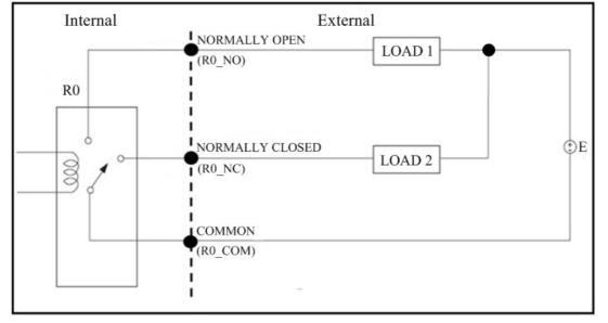
Figure 3.2 Relay Output Connection
