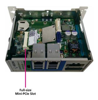
2. Push the module down and secure it with screws. Ensure the screws are fixed tightly to the slot.
