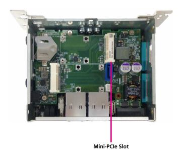
2. Insert the mSATA module into the mini-PCIe slot at 45 degree angle until the gold-plated connector on the edge of the module completely disappears into the slot.
