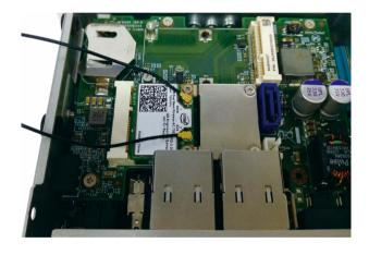
2. Locate the antenna holes on the top panel and insert the antenna jacks through the antenna holes. Fix the antenna jacks with ring 1 then ring 2.
