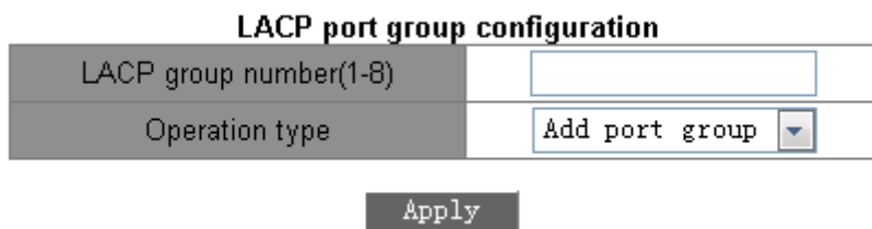
Figure 61 Port Channel Configuration
