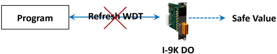
When Watchdog timeout occurs and `WDT_Overwrite = 0`, I-9K digital output values will all enter Safe Values, the operation for writing output value will not accept until reset Watchdog. If timeout occurs and `WDT_Overwrite = 1`, writing output value will be accept and Watchdog will be reset by writing output value.
