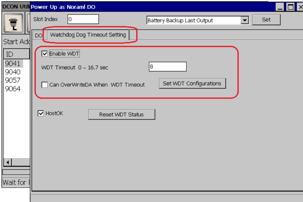
4. After setting, click “Set WDT Configurations” to save setting and the Watchdog will start counting until timeout or reset. If WDT timeout, system will reboot without power off, then the module will out save value. But if click “Reset WDT Status” before timeout, then the watchdog will recalculate
