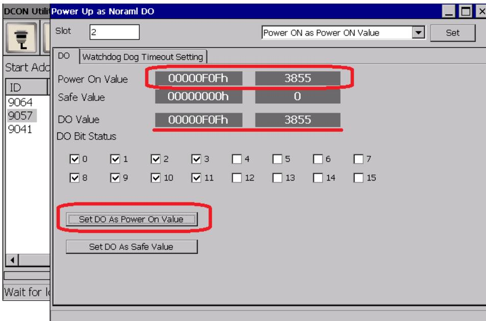
**4. Now you can reboot the system, the module will output the Power-on value when the Power on**
