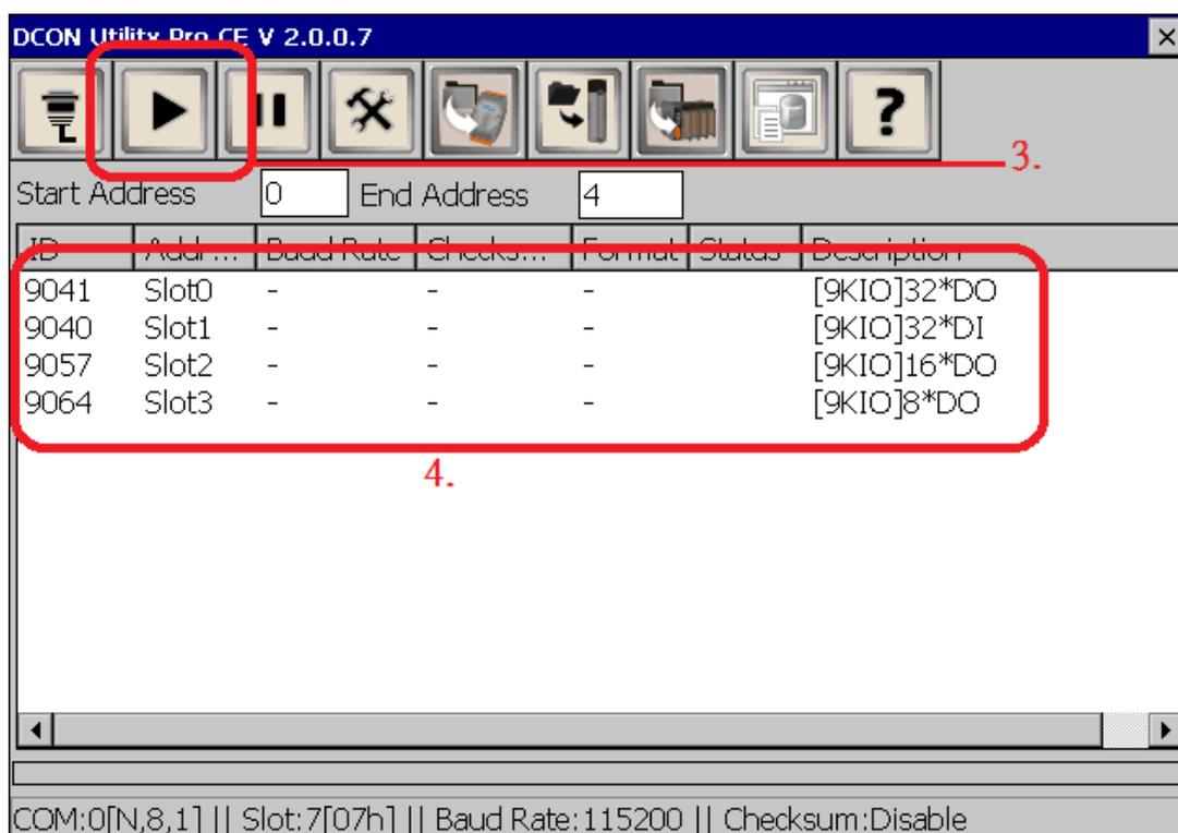
4. If any I/O devices are located, they will be displayed in the device list window
