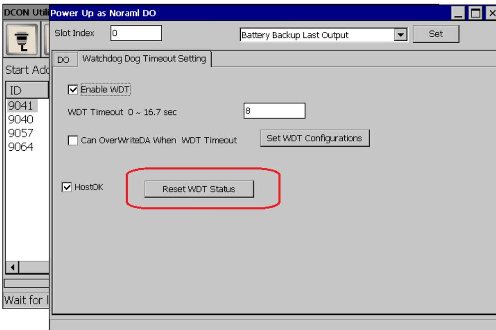
5. If “Can OverwriteDA When WDT Timeout” didn’t set to WDT configuration, then the module can’t output any value when the WDT start counting
