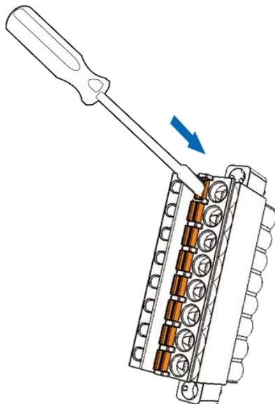
2. Remove the wiring from the terminal block
